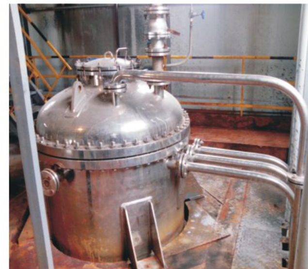
BG系列不锈钢管微孔过滤机 BGT series stainless steel microporous tube filter
