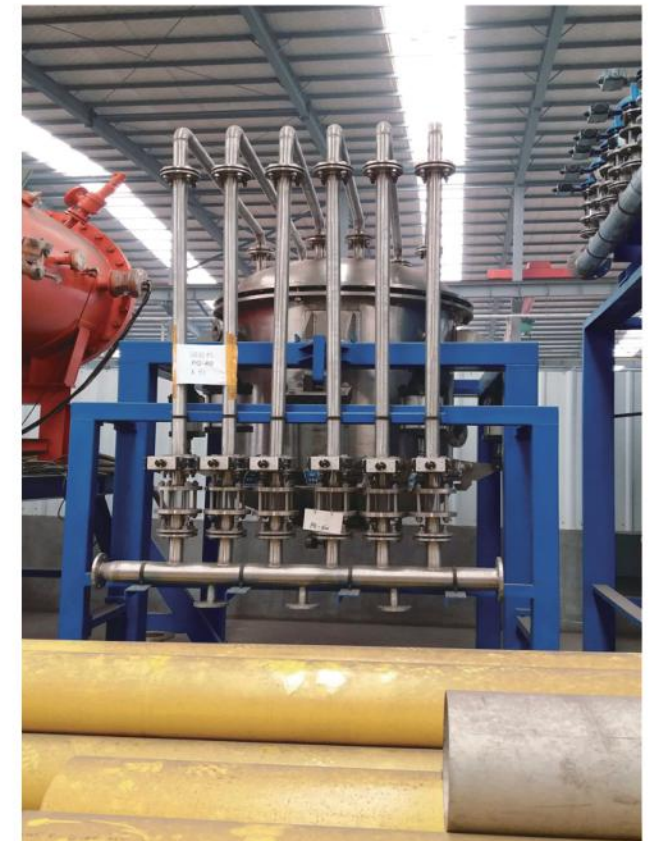
TGT系列陶瓷微孔过滤机 TGT series ceramic microporous tube filter
